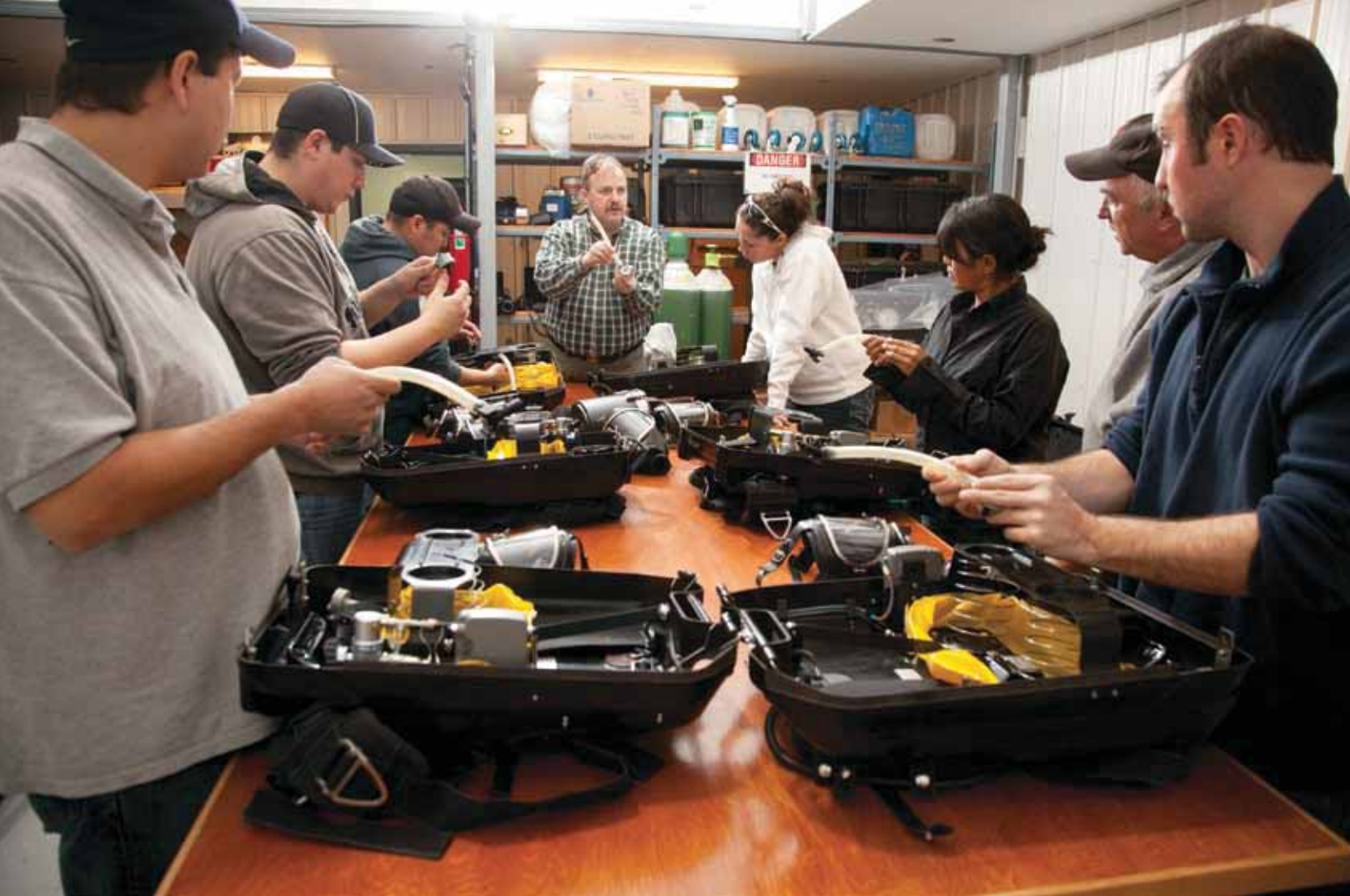
ABOVE: Underground mining students assemble and bench-test mine rescue breathing apparatus. RIGHT: A trainee in a diamond-driller helper program gets on-site experience.
